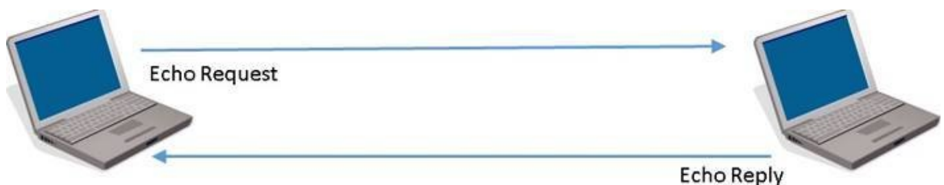
Figure 2: Echo Request and Echo Reply
