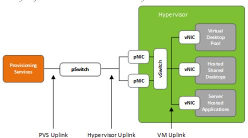
Figure 33: Sample PVS Network Configuration
