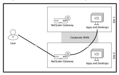
Figure 19: HDX Optimized Routing – Not Optimized
