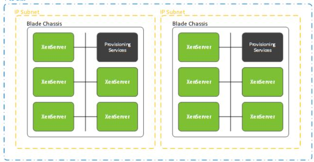
Figure 34: PVS Blade Enclosure Design
