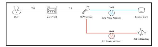
Figure 24: SSPR Architecture
