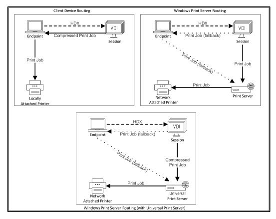
Figure 27: Auto-created and User-Added Print Job Routing
